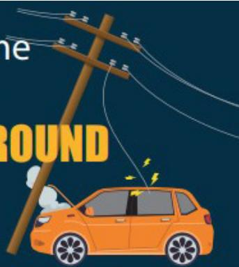
When electric utility equipment becomes damaged, the ground and objects can become energized.
